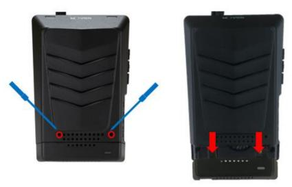
4 Unscrew two cross recessed screws marked in red to remove the Upper Back Cover.
