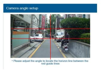
In case of indoor installation or somewhere you cannot see the horizon properly, use same data to "Camera Height". Mark the same height on the wall apart about  $3 \sim 5$  meters from the vehicle.
