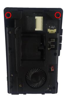
3 Remove PCB unit from mounting frame completely.
