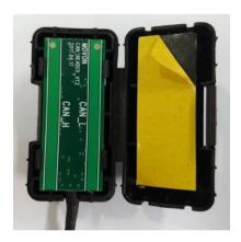
3 Attach the vehicle's CAN wire as straight as possible to the double-sided tape by aligning with the hole marked in red.
