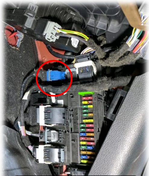
2016 F150: Blue connector at pass side BCM
